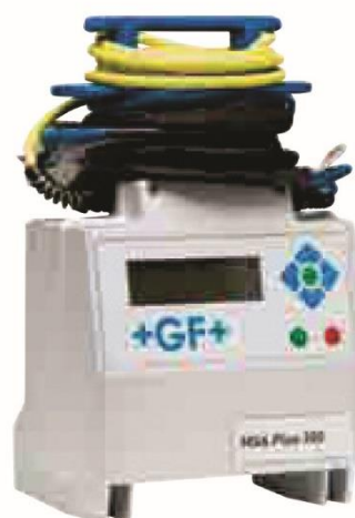
Figure 2- Typical Electrofusion Equipment
