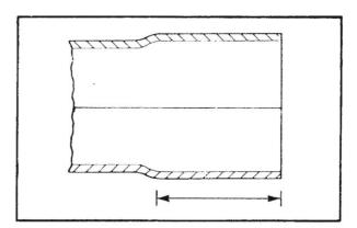
3 The mating areas of the spigot and socket should be thoroughly cleaned using the Watermain Cleaning Fluid provided and a clean rag or absorbent paper.
