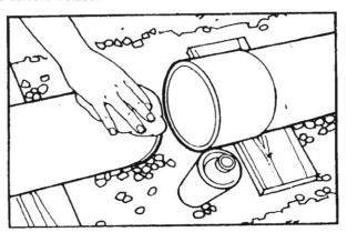
4 Lightly roughen the mating surfaces of the spigot and socket, using clean emery cloth or medium glass paper.
