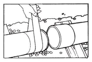
Thoroughly clean again the mating surfaces using the Watermain Cleaning Fluid provided and a clean rag or absorbent paper Ensure that all mating surfaces are clean and completely dry.
