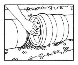
The spigot end and triple sealing portion of \_ the sealing ring should be lubricated with the Watermain lubricant supplied with the pipe. The spigot should be lubricated to the full insertion depth and around its complete circumference, paying particular attention to the chamber area. The triple seal should be lubricated around its complete circumference. The guiding principle should be to apply a liberal quantity of applicant and avoid dry areas on the mating surfaces.
