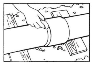
**8** Leave the joint undisturbed for five minutes, then handle with reasonable care. N.B. See Inspection and Testing, Page 29 (Thrust Forces Section).
