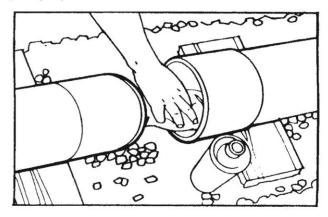
6 Using a brush of the size recommended - (see Page 33) apply an even layer of Watermain Solvent Cement to the spigot and socket mating surfaces The cement should be applied in a lengthwise direction and NOT with a circular motion. For joints of nominal diameter 3 and above, the cement should be applied simultaneously to the spigot and socket by two people.
