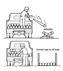
b) Where ever possible the loading and unloading of pipes should be carried out by hand. A six meter length of 10 nominal diameter PN 1 2 Watermain weighs 93 kilograms and can be carried by to men in normal site conditions.
